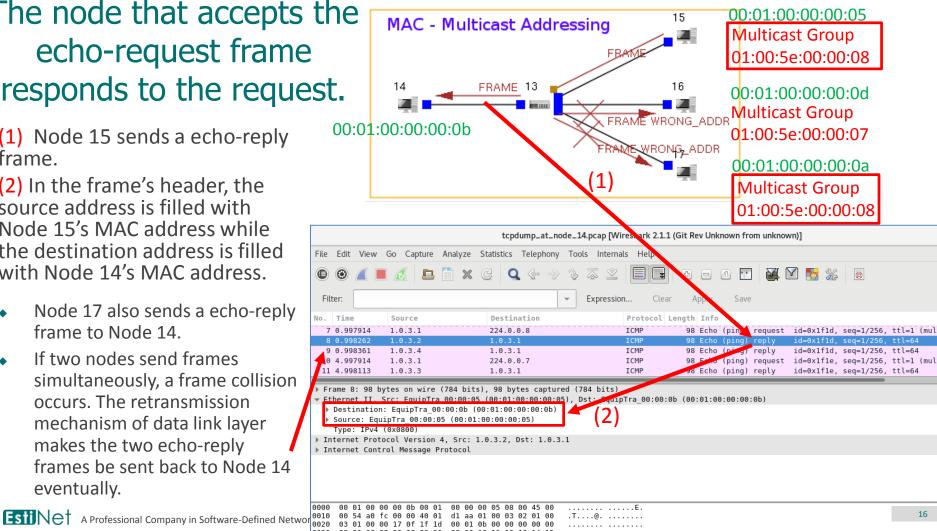
Fill the destination address of a data-link-layer frame with a multicast address to address those nodes that join a specific multicast group.
