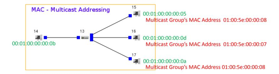
Fill the destination address of a data-link-layer frame with a multicast address to address those nodes that join a specific multicast group.
