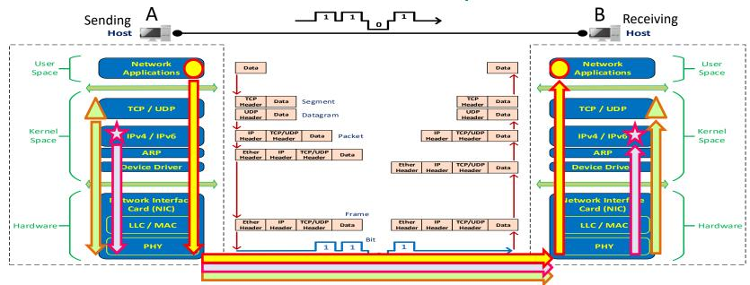
End-to-end Delay = Sending Host's Kernel/User Space Processing Delay (e.g., Protocol, Scheduling, Queuing, etc.)
