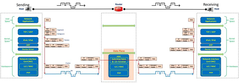
End-to-end Delay from Sending Host to Receiving Host
