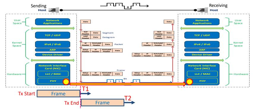
Sending Host's Interface Data Rate = X Mbps =  $(X * 10^6)$  bps Frame Size = Y bytes = (8 \* Y) bits Transmission Time = T2 - T1 =  $(8*Y)/(X * 10^6)$  sec
