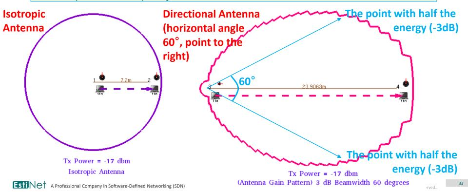
The transmission power of signal is gradually attenuated along with the signal emission path. When the power is lower than the receiving sensitivity of a receiver, no signal is received.
